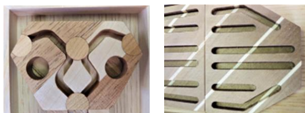
図14 裏面の溝彫・穴彫加工
