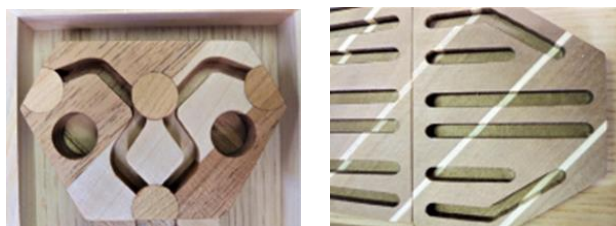
図14 裏面の溝彫・穴彫加工
